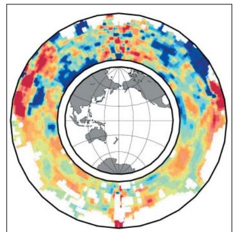
Fig. 1. Holes in the mantle: An example of poor resolution of mantle structure in the Southern Hemisphere and elsewhere due to the absence of seismic stations in the oceans. A polar cross section through a *P* wave speed anomaly model [van der Hilst *et al.*, 1997] shows undersampled regions in white [Boschi and Dziewonski, 1999].
