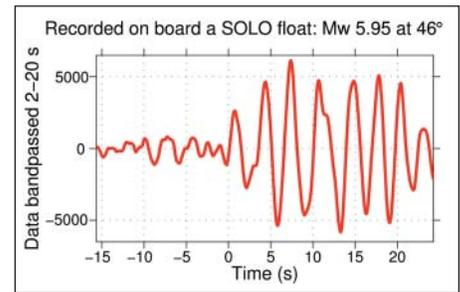
Fig. 3. The clear onset of a P wave from a magnitude 6.0 earthquake at a distance of 46 degrees detected by the hydrophone on board the experimental MERMAID float on its trip adrift 700 meters below the sea surface. The waves from this teleseismic earthquake have sampled a hitherto uncharted volume of the Earth's mantle.
