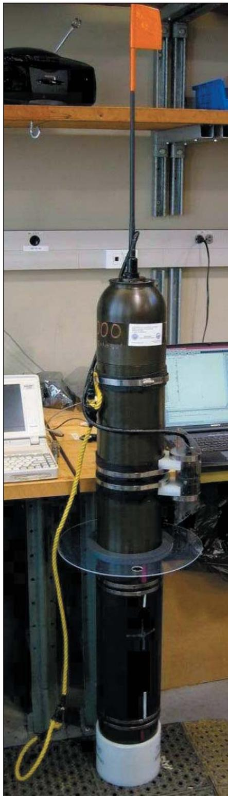
Fig. 2. The MERMAID prototype. The hydrophone protrudes from the middle right. Thousands of similar drifters, though none capable of detecting earthquake signals, are currently afloat the seven seas in an effort to map the temperature and salinity of the upper 2000 meters of the ocean.
