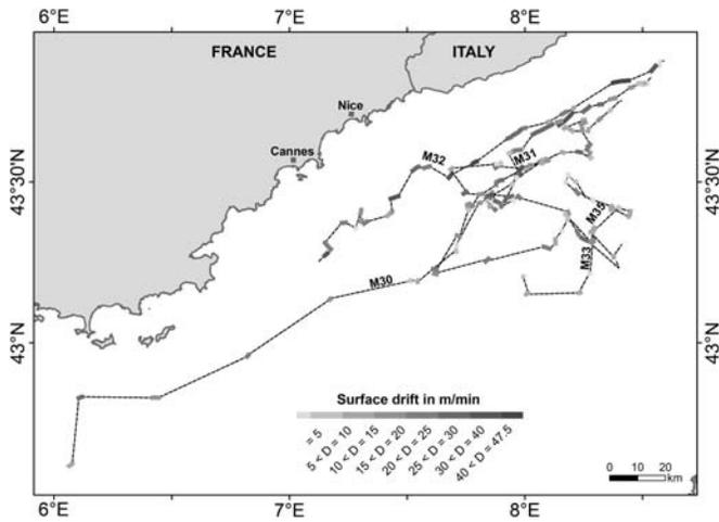
▲ **Figure 2.** The trajectories of floats used in the experiment are shown. Thick lines indicated surface drift (in meters per minute) with velocity in grayscale. MERMAID floats are labeled M30–M33 and M35.
