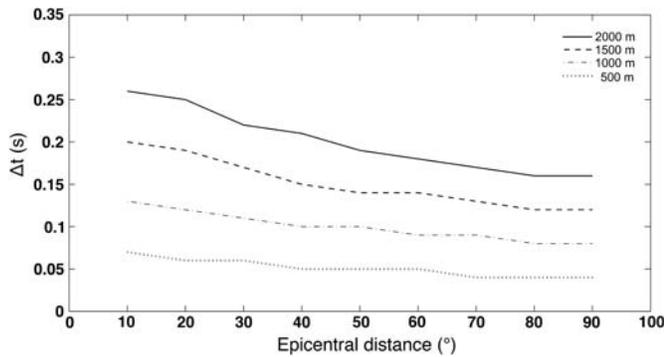
▲ **Figure 5.** Equivalent time errors (in seconds), as a function of the epicentral distance of an earthquake, in the case of a record without an immediate surfacing. The curves represent four typical locations errors (500, 1000, 1500, and 2000 m).
