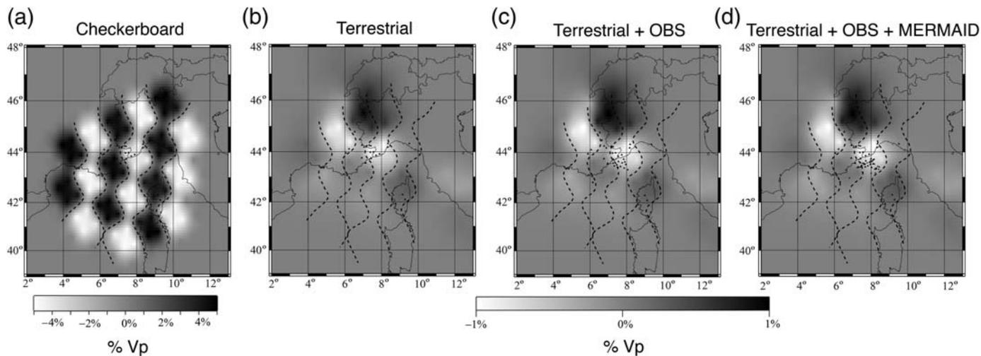
▲ **Figure 8.** Checkerboard resolution tests based on  $156 \times 156$  km anomalies at 226 km depth. (a) The checkerboard used with  $\pm 5\%$  velocity anomalies, (b) the solution obtained with data acquired with terrestrial stations only, (c) solution obtained with terrestrial and GROSARIN OBS stations, and (d) the solution obtained with the two previous datasets and MERMAID floats data. The dotted black curves correspond to the limits between illustrated cells in (a).
