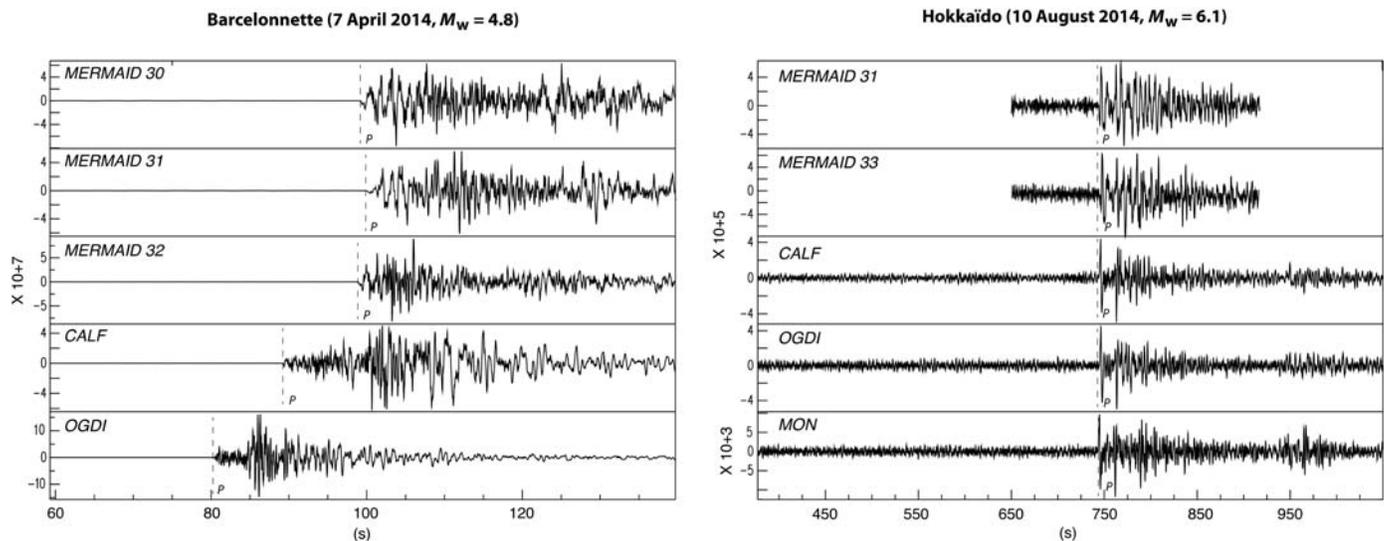
▲ **Figure 6.** Regional Barcelonnette (France, 7 April 2014,  $M_w = 4.8$ ) and teleseismic Hokkaïdo (Japan, 10 August 2014  $M_w = 6.1$ ) earthquakes recorded by MERMAID floats and terrestrial permanent stations. The locations of stations are illustrated in Figure 1. The time axis is in seconds and begins at 19:25:45 for the Barcelonnette earthquake and at 03:43:20 for the Hokkaïdo earthquake. The amplitude axis is in counts.
