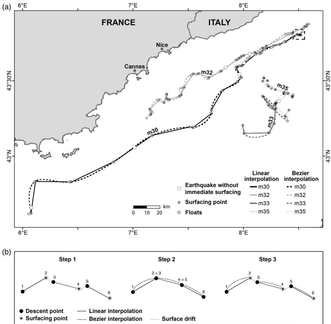
▲ **Figure 4.** (a) Bézier interpolation trajectories of MERMAID floats during an earthquake recording without an immediate surfacing (open circles). Linear trajectories of MERMAID floats are in solid curves and Bézier interpolations are in dotted curves. (b) Interpolations corresponding to the Bézier interpolation principle (see text).
