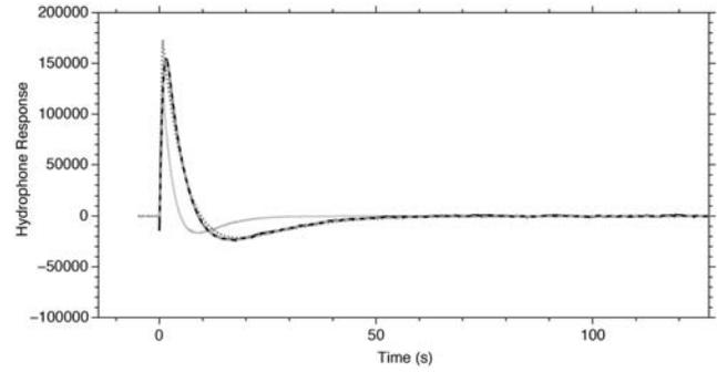
**Figure 5.** The step response of the MERMAID system (black curve) and the final fit for four poles and three zeros (dashed gray curve). The starting fit (using equation 7, with two poles and one zero) and the result of the first iteration are given by the light gray and the dotted gray curves, respectively.
