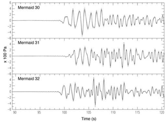
**Figure 7.** Instrument-corrected MERMAID records of the Barcelonnette earthquake for different values of  $t_\tau$ : the dashed black signal for  $t_\tau = 0.65$  s, the black signal for  $t_\tau = 0.73$  s, and the dotted gray signal for  $t_\tau = 0.80$  s.
