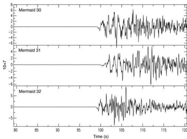
**Figure 1.** Raw digitizer output of the Barcelonnette earthquake ( $M_w$  4.8) recorded by three Mobile Earthquake Recorder in Marine Areas by Independent Divers (MERMAIDs) on 7 April 2014. The time axis is in seconds and begins at 19:25:45 UTC. The amplitude axis is in counts.
